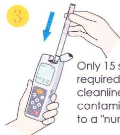
Only 15 seconds are required to measure the cleanliness. Invisible contamination changes to a "numerical value."
